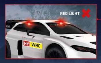
A flashing red light, along with an alarm sound, means the car is unsafe. No light means it is potentially unsafe. Only touch the car if there is a green light.
