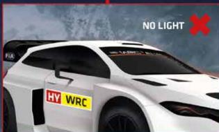
2 Safetylights are on the windscreen and both side pillars of the cars. Following an accident, a solid green light means it is safe to touch.
